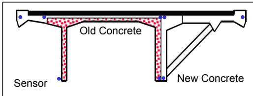
Figure 3: Position of sensors in cross-section
