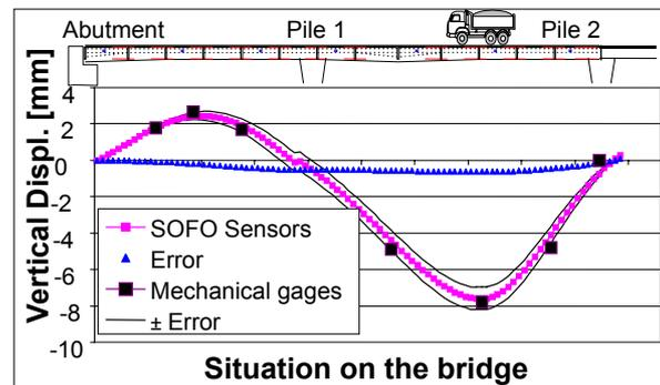
Figure 6: Monitoring during the load test
