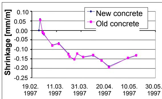
Figure 5: Old-new concrete interaction monitoring
