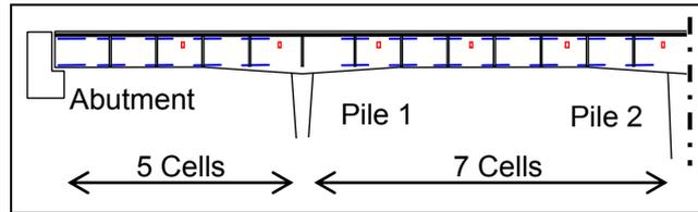
Figure 4: Longitudinal position of sensors
