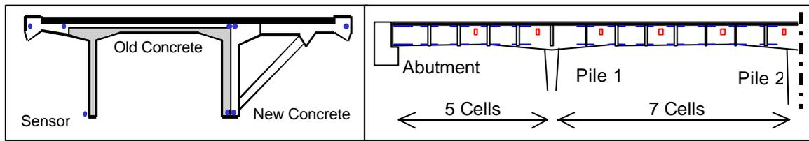
Figure 6: Old-new concrete interaction monitoring
