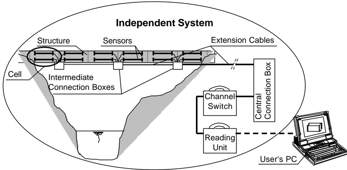
Figure 2: Parallel topology used for structural monitoring and difference between long-gage structural monitoring and short-gage local material monitoring
