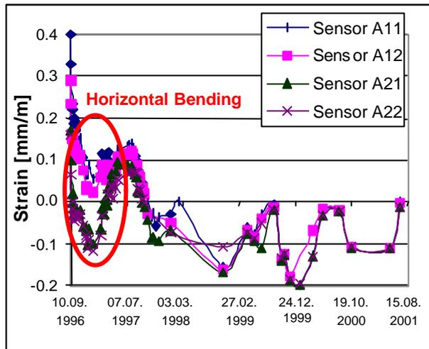
Figure 9: Uncoupling of shrinkage and temperature
