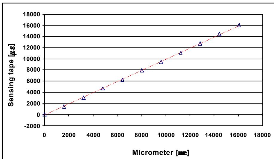
Figure 9: Linearity between micrometer and sensing tape measurement (for rising load only)
