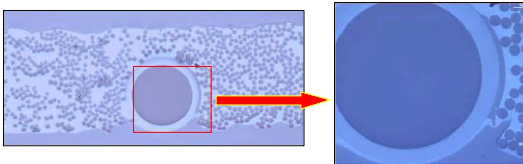
Figure 6: Optical fiber emerges from the tape at bottom of the cross-section; delamination is observed in close up.
