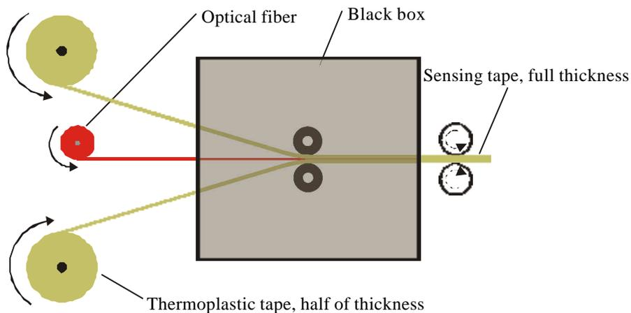
Figure 3: Production of the sensing tapes using the “sandwich” technique
