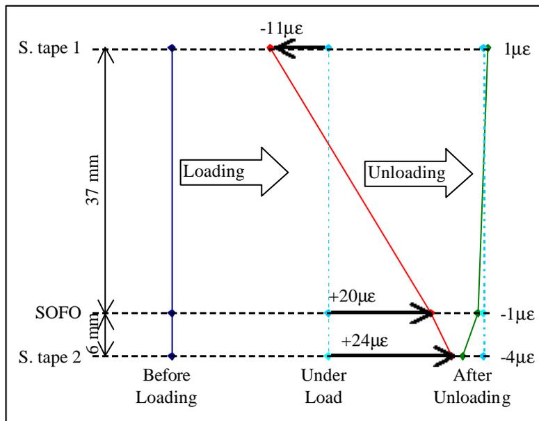
Figure 11: Results of the rail test using the sensing tapes and standard SOFO sensor
