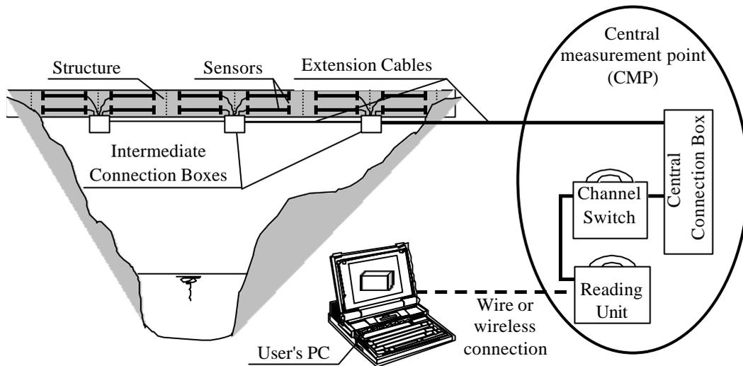
Figure 1: Components of the SOFO system
