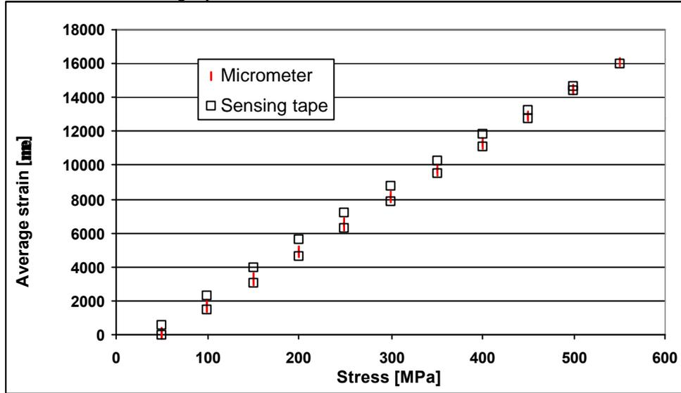
Figure 8: Strain-stress diagram of the sensing tape obtained using both, micrometer and sensing tape as a SOFO sensor
