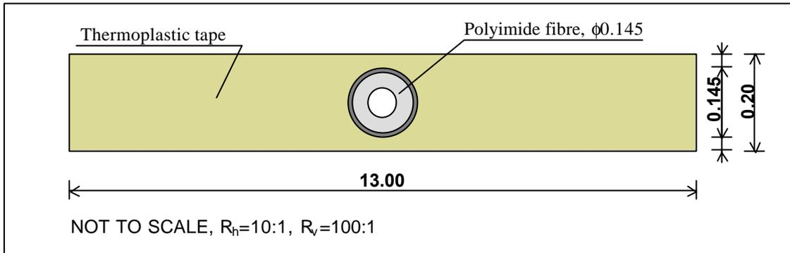
Figure 2: Cross-section of the sensing tape
