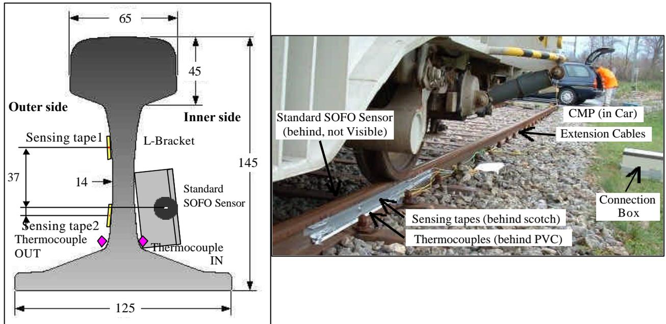
Figure 10: Position of sensing tapes and standard SOFO sensor installed on rails, and photo taken during the test
