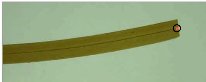
Figure 4: Sensing tape with inserted visible light (encircled)
