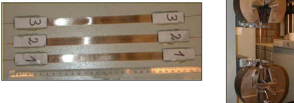
Figure 7: Sensing tape samples before the test (left) and set-up for traction (right).
