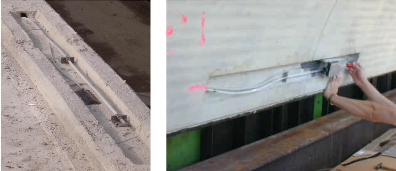
Fig. 4: Resistive and fibre-optic strain gages in a depression on the surface of the concrete bridge before embedding.
