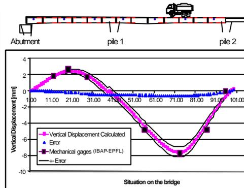
Figure 7: Vertical displacement during the load test and comparison with dial gages
