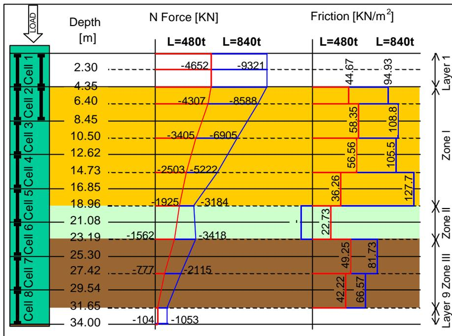
Figure 4: Sensor network and main results obtained using simple topology for pile monitoring
