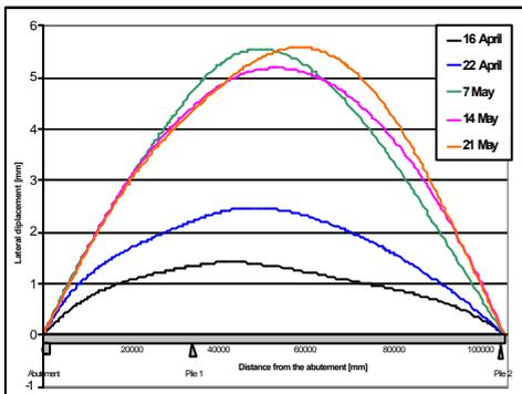
Figure 6: Horizontal displacement evolution due to new concrete shrinkage
