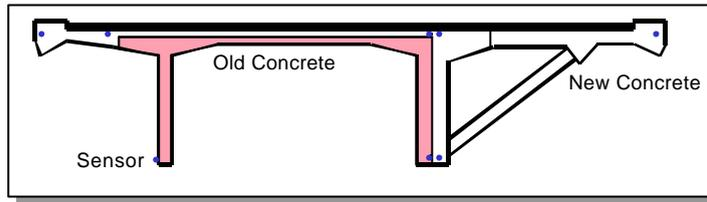
Figure 5: Position of sensors in cross-section of Versoix bridge
