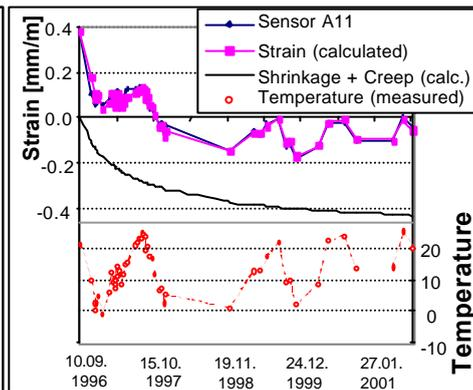
Figure 9: Uncoupling of shrinkage and creep from temperature
