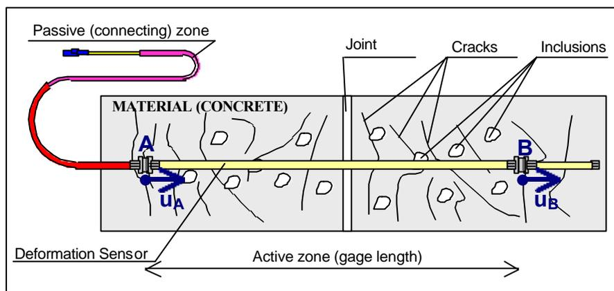
Figure 1: Schema of a long-gage sensor installed on a material with cracks, inclusions and joints (e.g. concrete)
