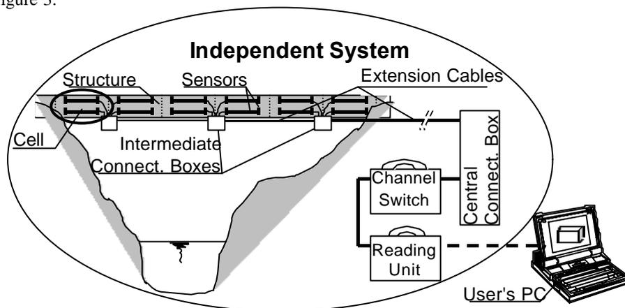
Figure 3: Typical application and components of the SOFO monitoring system
