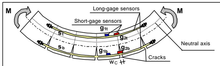
Figure 2. Difference between material and structural monitoring and parallel topology of long-gage sensors
