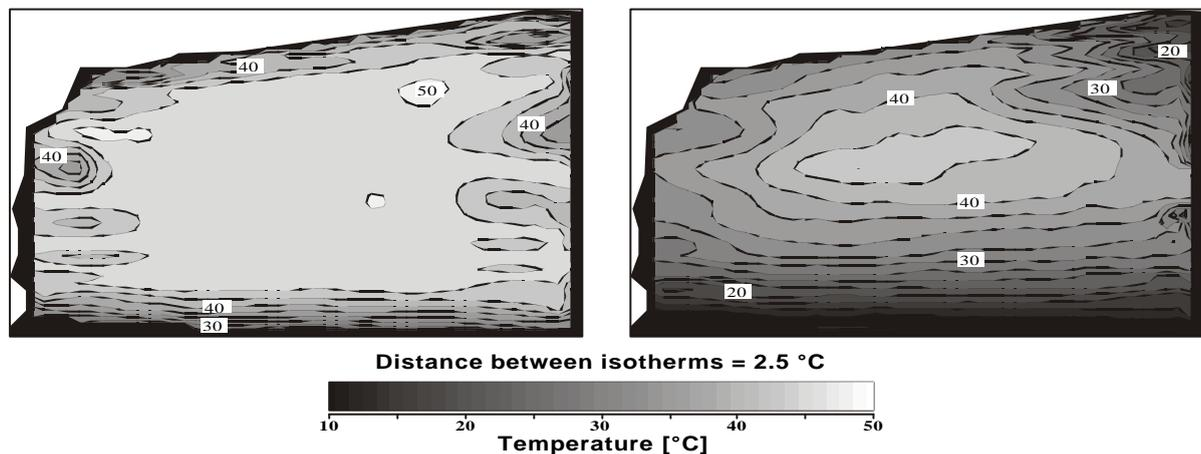
Fig. 2 Luzzone Dam: Temperature distribution measured with the DITEST system 15 and 55 days after concrete pouring (Courtesy of L. Thévenaz and P. Robert, MET-EPFL, Switzerland)
