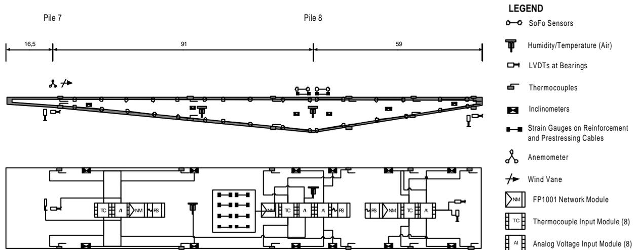
Fig. 5: Partial instrumentation scheme for one girder box
