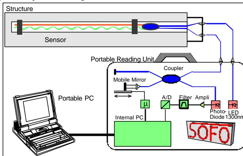
Fig. 2: Schema of functioning and components of the SOFO system
