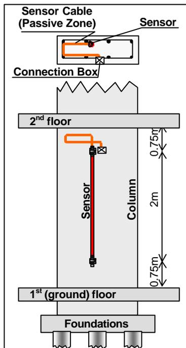
Fig. 3: Sensor position in column
