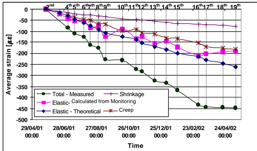
Fig. 7: Evolution of strain components obtained from modeling and monitoring, and evolution of theoretical elastic strain for column C3.
