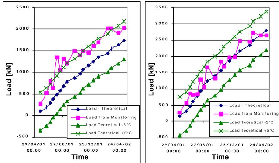
Fig. 8: Evolution of load in columns C1 and C8 – comparison between theoretical values and values obtained from monitoring
