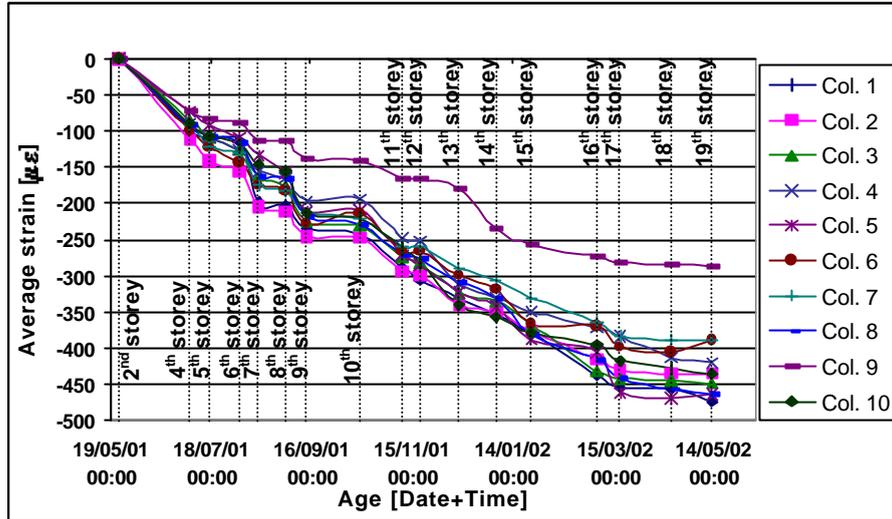
Fig. 6: Evolution of total average strain in columns monitored by SOFO system
