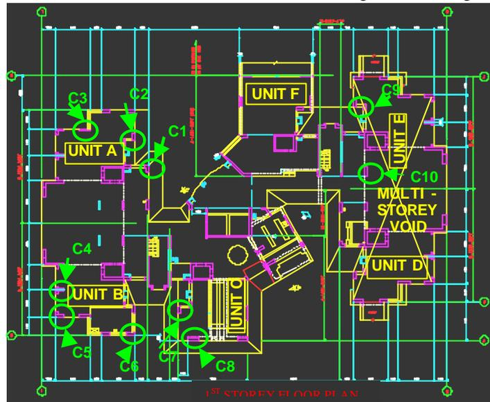
Fig. 5: Position of the columns in ground floor equipped with sensors
