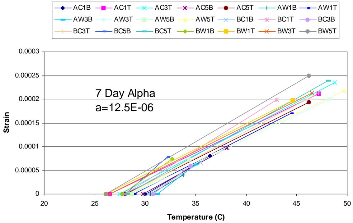
a. Coefficient of thermal expansion at 7 days
