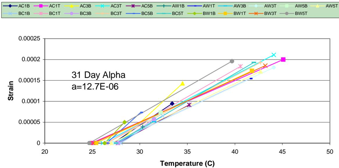
b. Coefficient of thermal expansion at 31 days
