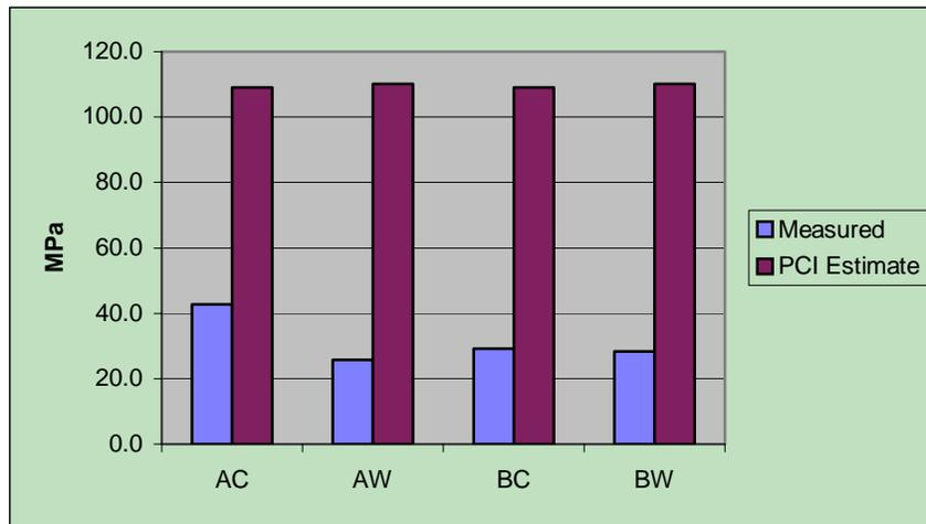
b. Prestress losses during storage for each beam
