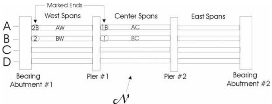
Figure 4. Plan View of the bridge showing the monitored beams
