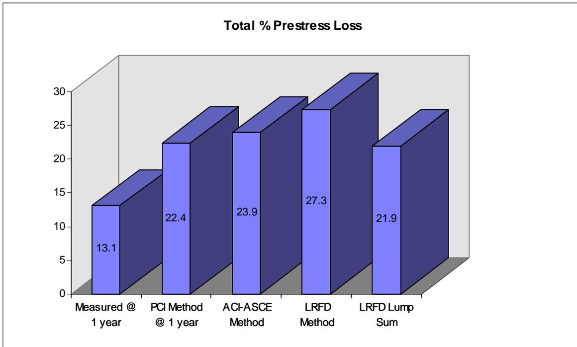
Figure 9. Measured losses vs. losses estimated by various methods
