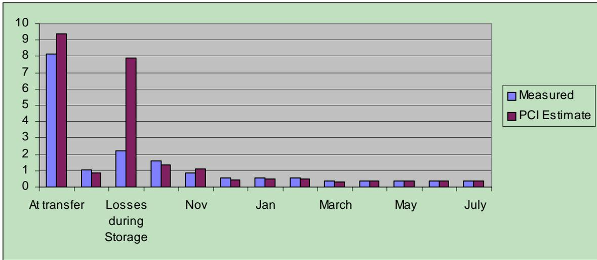
Figure 8. % prestress loss. Field measurements vs. the PCI Method
