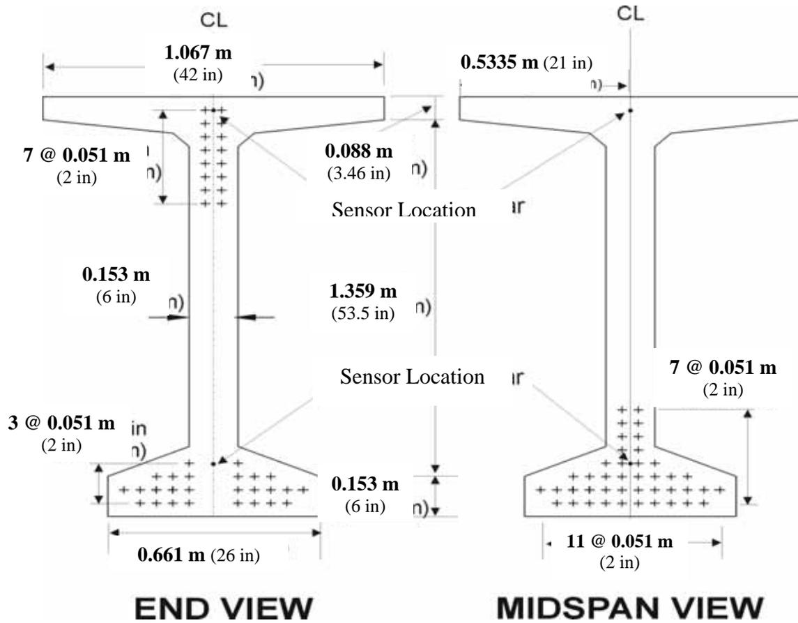
Figure 3. Cross-sectional view of BT-1600 I-beam
