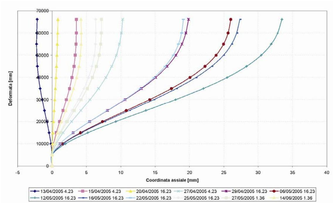
Figure 3. Deformed shapes of the pylon
