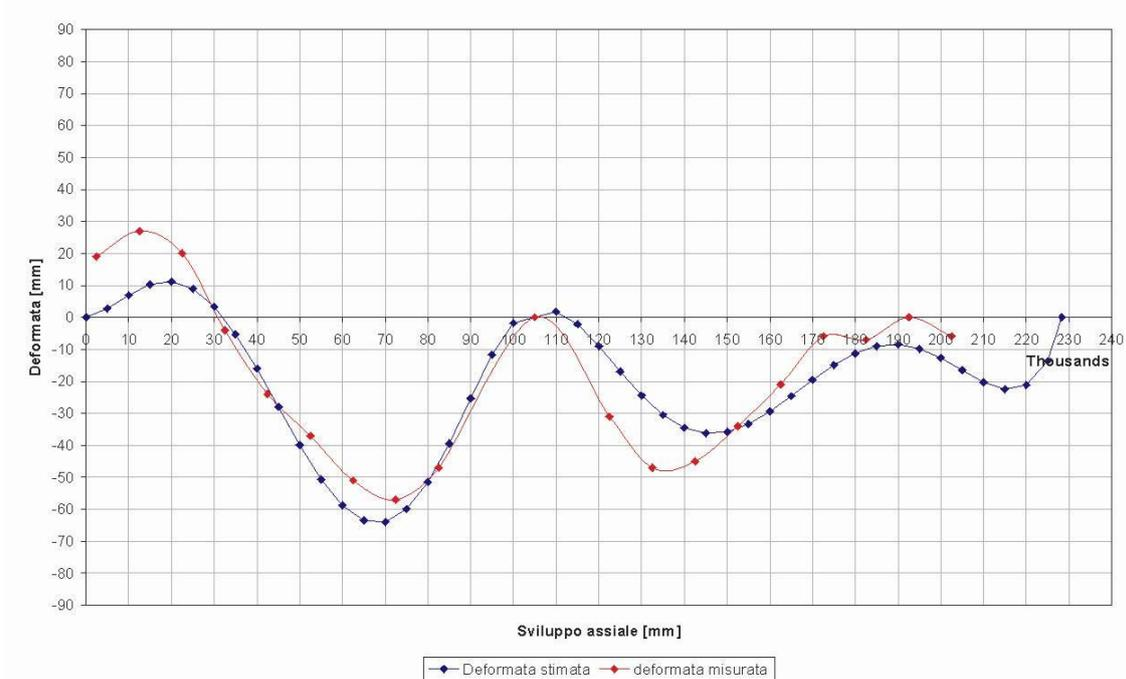
Figure 2. Comparison between the evaluated deformed shape and topographic measures
