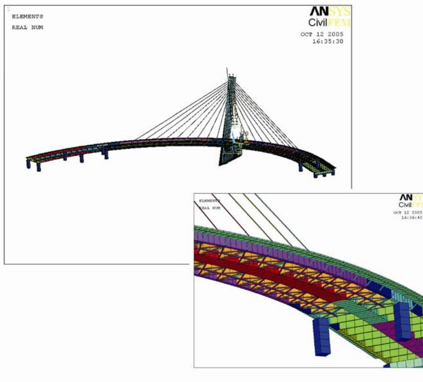
Figure 4. Finite-element model of the bridge
