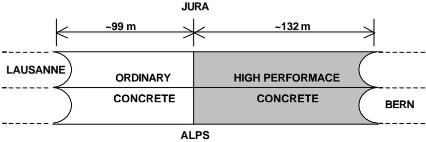
Figure 4: Simplified Plan View of the Cut-and-cover Tunnel of Champ Baly
