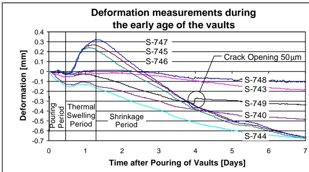
Figure 7: Deformation Measurements at the Early Age of the Vaults
