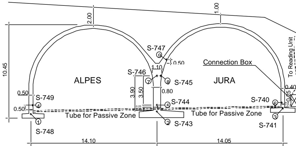
Figure 5: Cross-section of the Tunnel and Sensor Placement
