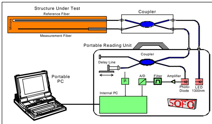
Figure 1: Set-up of the SOFO System
