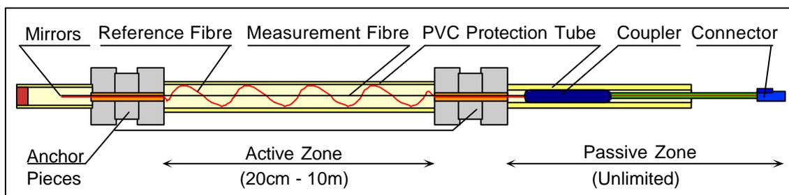
*Figure 2: Schema of a SOFO Standard Sensor*
