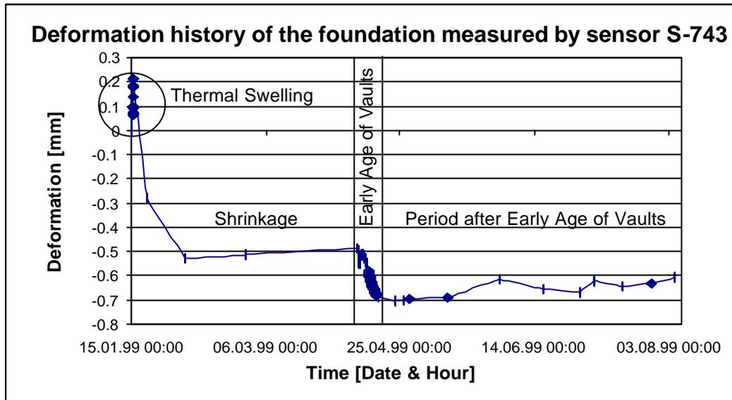
Figure 6: Long-term Deformation Measurements of the Foundations
